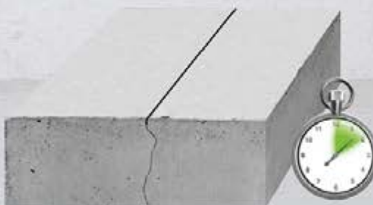
Soff-Cut has the Ultra Early Entry™ dry-cutting system which controls random cracking by making the cut at an early stage.
