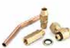
13 Supplementary cooler, to be used where the inlet water temperature is higher than 25°C or the outlet water flow from the machine is lower than 5 l/min
