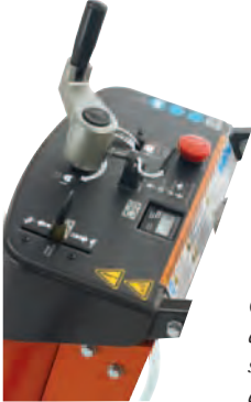
Comprehensive console with engine throttle, emergency stop switch, tachometer, timer and depth indicator.
