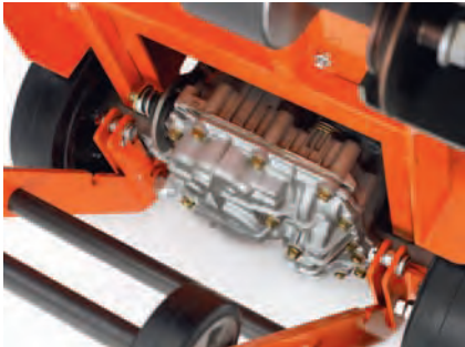
Self-contained differential drive system eliminating drive gear from rear wheels and related wear. It is simple to handle and maintain.
