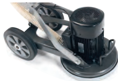
The efficient suction of grinding dust is a result of the design of the dust guard and vacuum port.
