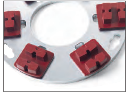
Low-profile disc holder with recessed locking mechanism reduces overall height of tooling, increasing the efficiency of dust extraction.
