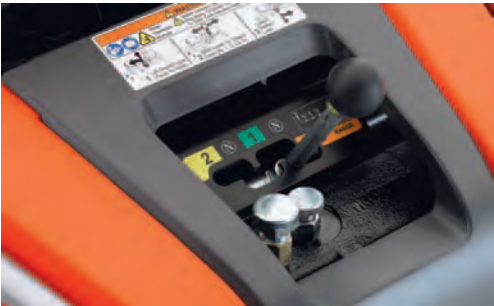
The gearbox shift lever is used to change the output speed of the engine gearbox. Three speeds and two neutral positions are standard. The gearbox shift lever positions are colour-coded to match the blade diameter and the bladeshaft rpm decal located on the control panel. Gearbox detent locks the gearbox shift lever in position.
