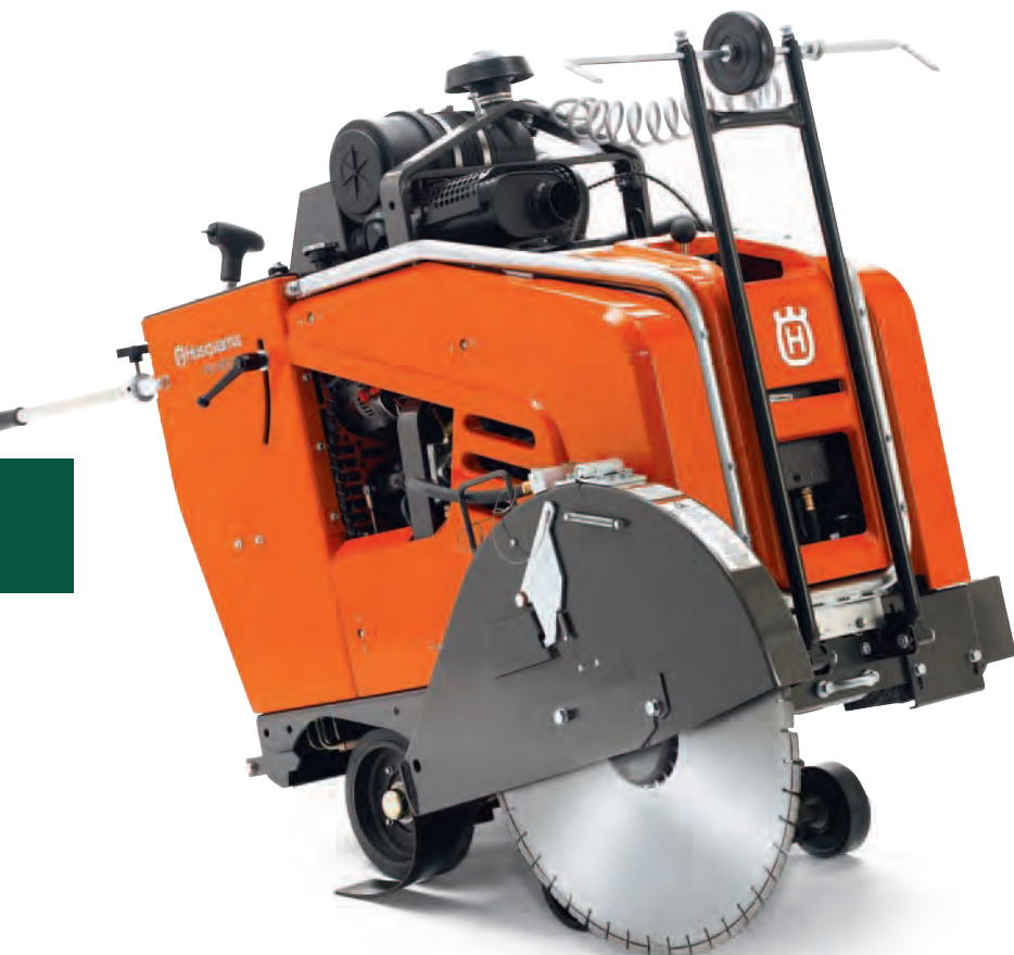
The tachometer/blade shaft rpm gauge indicates engine rpm or blade shaft rpm. Blade shaft rpm range is colour-coded to gear selection position.
