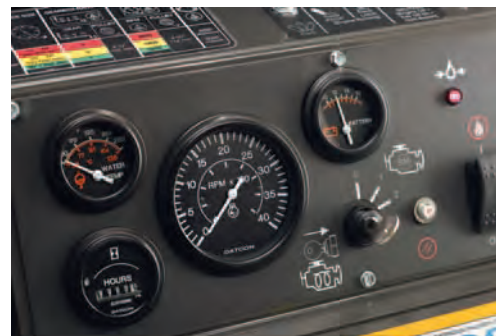
The tachometer/blade shaft rpm gauge indicates engine rpm or blade shaft rpm. Blade shaft rpm range is colour-coded to gear selection position.
